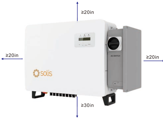
Figure 3.2 Clearance distances requirement for the inverter
