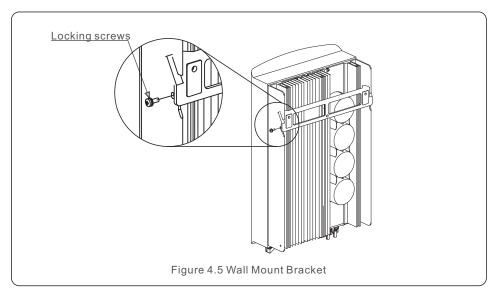
5. Use M4\*9 screws in accessory to lock the inverter to the mount bracket.
