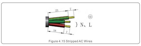
2. Fix the wires into the correct postion. Torque 0.8N.m
