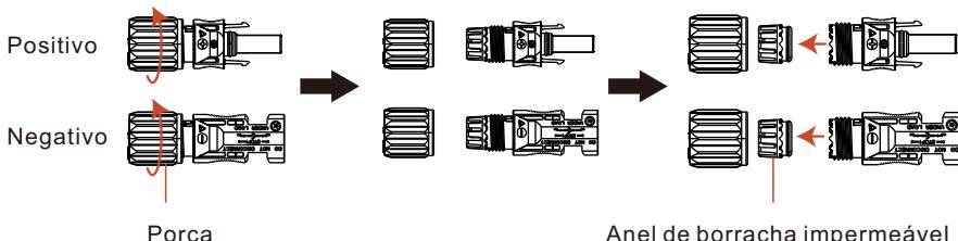
Figura 5.11 Remova a tampa do conector do terminal
