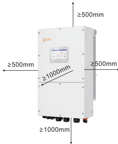
Figure 3.5 Inverter Mounting Clearances
