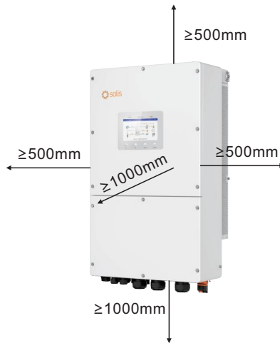
Figure 3.5 Inverter Mounting Clearances
