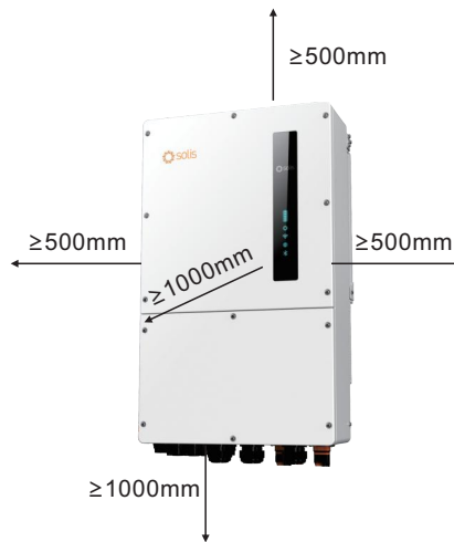
Figure 3.5 Inverter Mounting Clearances
