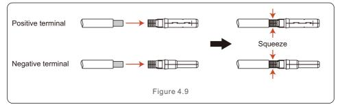
5. Insert the crimped DC cable into the DC terminal firmly, then insert the waterproof rubber ring into the DC terminal and tighten the nut.
