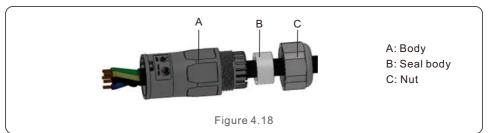
3. Crimp wires, screw torque 0.8N·m±0.1N·m.
