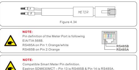
Eastron SDM630 – Pin B is RS485B & Pin A is RS485A.
