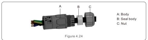
3. Crimp wires, screw torque 0.8N·m±0.1N·m.
