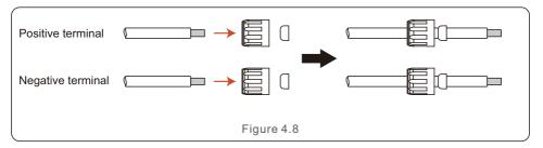
4. Connect the wire part of the DC cable to the metal DC terminal and crimp it with a special DC terminal crimping tool.
