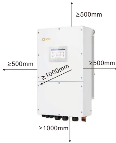
Figure 3.5 Inverter Mounting Clearances
