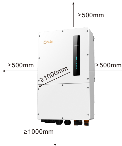
Figure 3.5 Inverter Mounting Clearances
