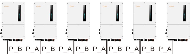
Figure 3.23 Parallel Terminal Connection
