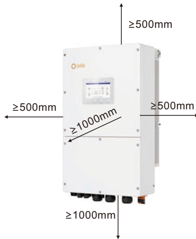
Figure 3.5 Inverter Mounting Clearances
