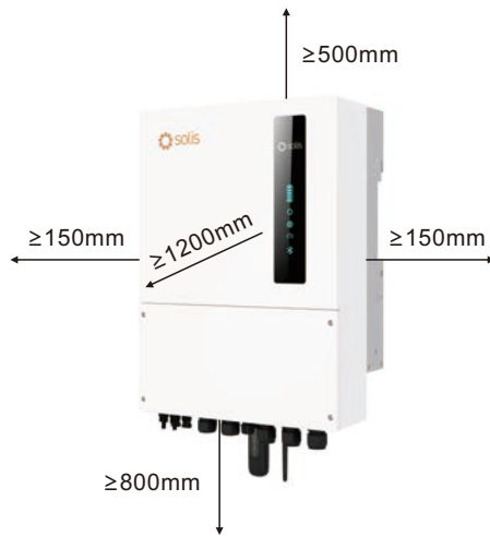
Figure 3.5 Inverter Mounting Clearances
