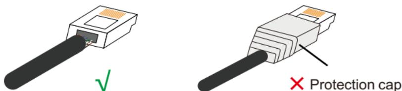
The diameter of the network cable connection end on the data logger is about 3.5mm after it is completely fastened. The network cable is required to be circular or oval, and the diameter of the network cable needs to be greater than 4mm in order to be properly sealed.
