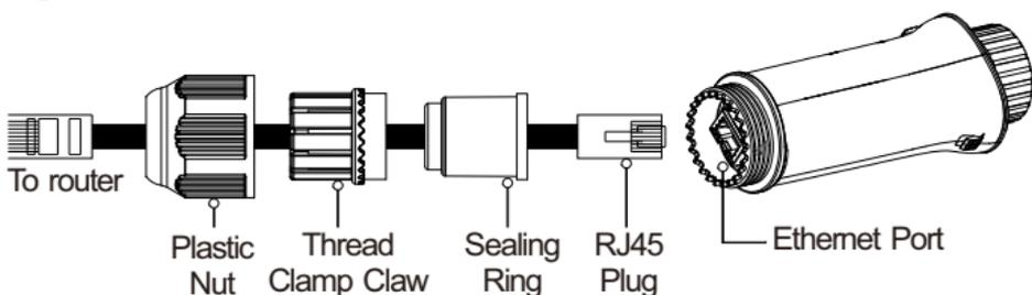
Step3: Fully embed the “Sealing Ring” into the “Thread Clamp Claw”.
