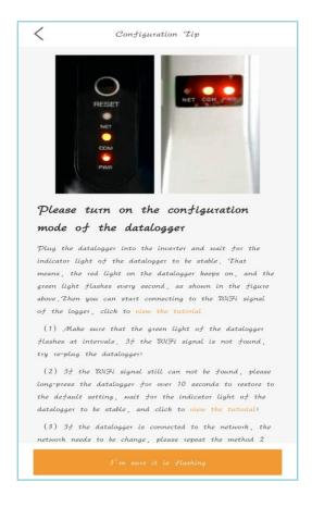
Step6: Connect the data-logger network, click [to connect], go to the network setting on your phone, choose the data-logger network.
